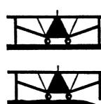
On uneven surfaces, one or more legs may not rest on the ground. It is recommended that the table is moved to a more level surface or else wedge the legs.
